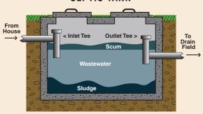
Incoming solid matter sinks. Soap and grease float. The tank has an outlet baffle to hold in undigested waste. Only clean water should leave the tank and enter the lateral pipes.
