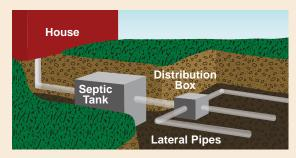
Septic tanks are designed to allow bacteria and enzymes to biodegrade organic waste. This amazing process actually converts waste into water, carbon dioxide and small amounts of mineral matter!
