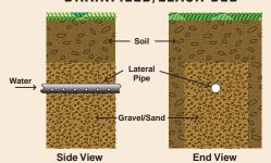
Water flows out of the laterals into a bed of gravel or sand which acts as a final filter before the water enters the ground.
